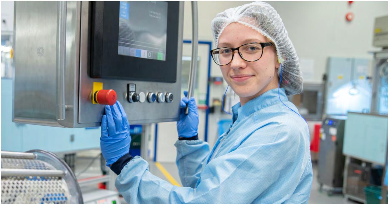
As one of the world's largest manufacturers of medical check valves Bespak by Recipharm uses high-speed automated equipment to produce high quality products. Each valve is 100% function tested as part of the assembly process to maintain our defect level of below 1 part per million.
